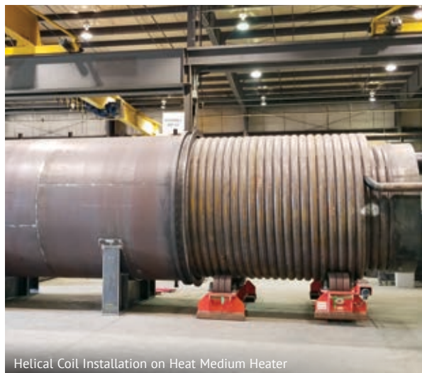
Helical Coil Installation on Heat Medium Heater
