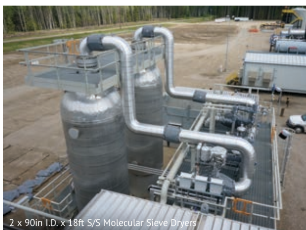
600 gpm Amine Gas Sweetening Train, 150 MMSCFD
